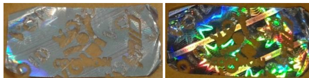
Figure 8.3 view of broken metrological mark
