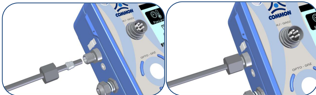
Figure 5.11 The connection of the pressure measurement to the P1 pressure sensor
